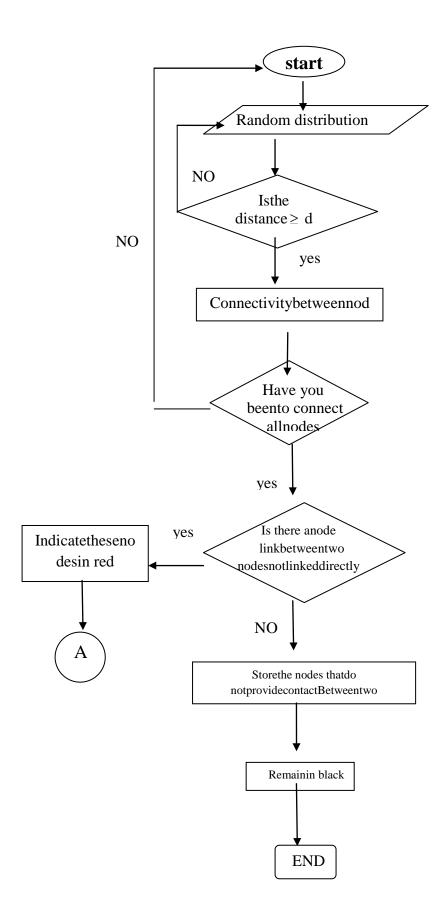
Figure 5. Flowcharttosimulatethe Basic Rule
